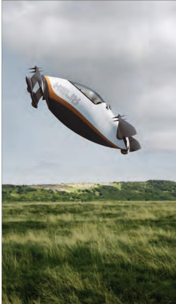
*In hover mode, all propellers point upwards.*
