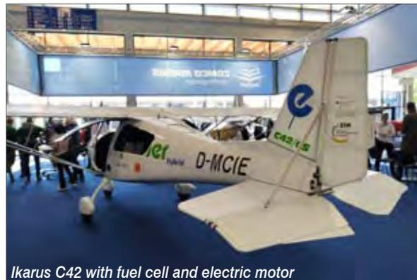
*Ikarus C42 with fuel cell and electric motor*
