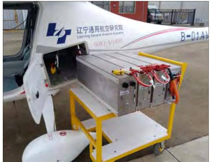
All RX series airplanes have removable batteries for continuous operation and upgrade potential. Shown here are the batteries of RX1E-A.
