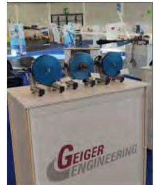
Geiger's 60 volt motors power a wide variety of ultra-light aircraft: from the small trike to the UL glider Wing from AIR and the two-seater Elektra Trainer.
