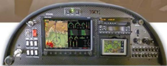
New instrument panels are available with modern avionics to meet your requirements
